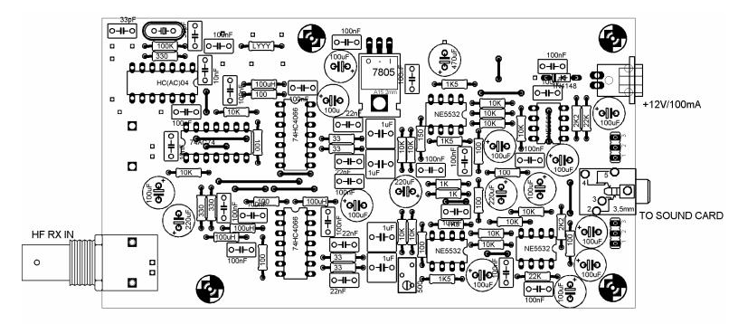
DR2A+ parts placement for crystal oscillator in overtone mode (one of two possible connections)
