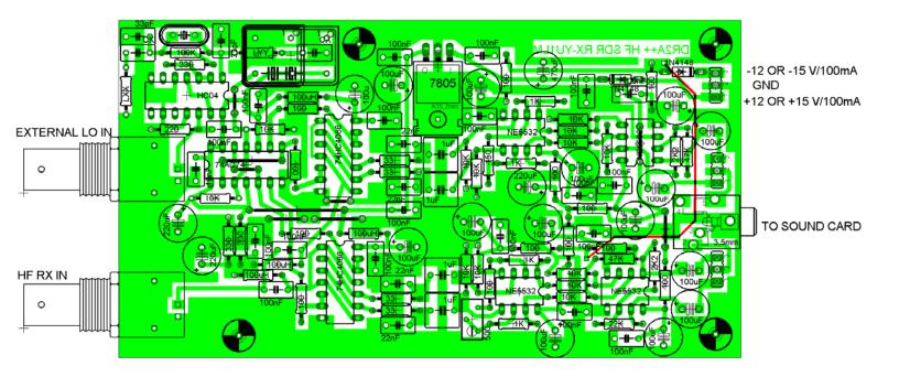
DR2A++ Single side PCB size is 133 x 73 mm, red wire at bottom side is -Vcc power connection
