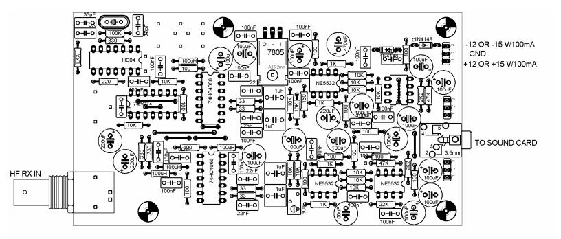
DR2A+ parts placement for crystal oscillator in overtone mode to 80-120 MHz with AC04 (one of two possible connections)
