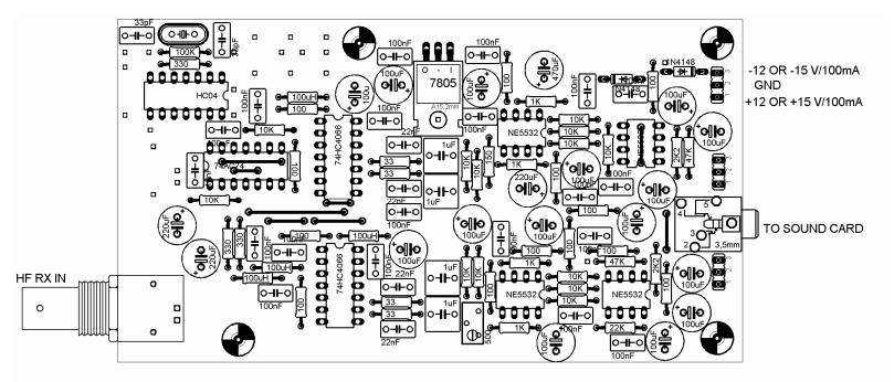
DR2A++ parts placement for internal crystal fundamental mode oscillator to 30 MHz or 3 overtone mode oscillator typical case Q=28322kHz (reduce 100K in HC04 feedback to 4k7)
