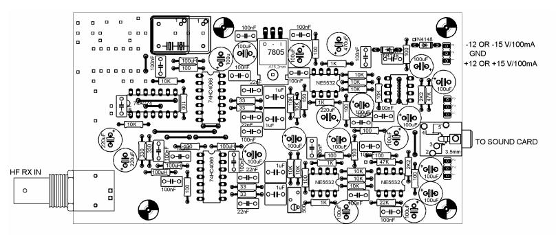
DR2A++ parts placement for the block oscillator
