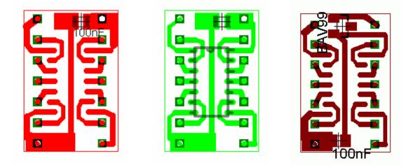
Single side SMT adapter PCBs (for 74LVC4066 and 74LVC74 right) top view dimensions are 21 x 11.5 mm
