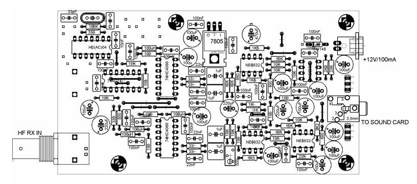
DR2A+ parts placement for crystal oscillator in fundamental mode (for 3 overtone reduce 100K to 4K7)
